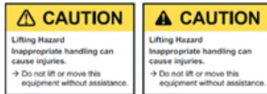
Fig. 6-4: Example: Notice in signal word panel
